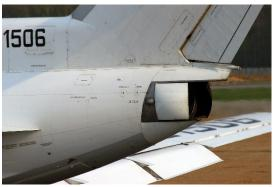
Bucket thrust reverser on the center engine
